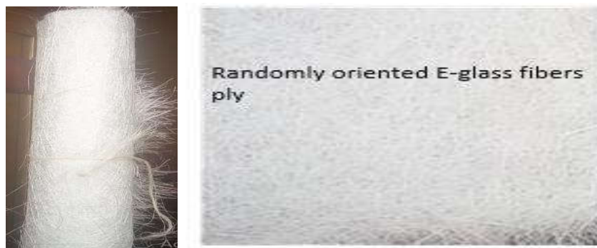
Figure 5. Randomly oriented glass fibers.
