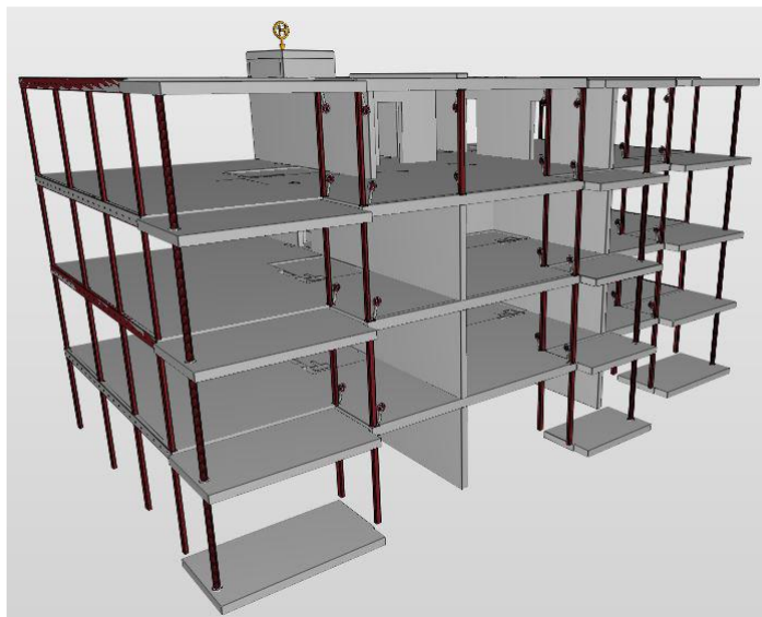
Figure 2. 3D model of considered apartment building
