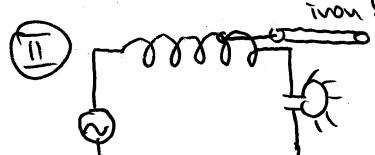
Assume sinusoidal power source. When iron bar B field inside solenoid increases,  $L$  increases what happens to brightness of bulb?
