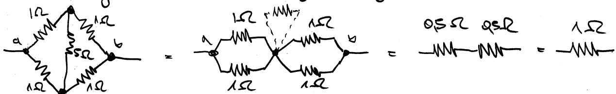
Since all resistors  $1\Omega$  on outside  $I_{ac} = I_{ad} \Rightarrow \Delta V_{ac} = \Delta V_{ad}$
