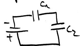
in series: charge flows onto  $C_1$  same as on  $C_2$ . Total potential difference must be the sum (Kirchhoff)
