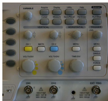
(b) Buttons and control knobs on the oscillator panel.
