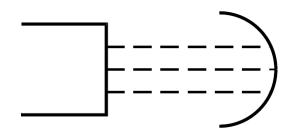
Select the semi-circular curved mirror. Aim a set of parallel rays into the centre of the inside curve of the mirror so that the rays are parallel to the axis of symmetry of the mirror. Record the incident and reflected rays and note where they meet. This point is called the **FOCUS** of the mirror.
