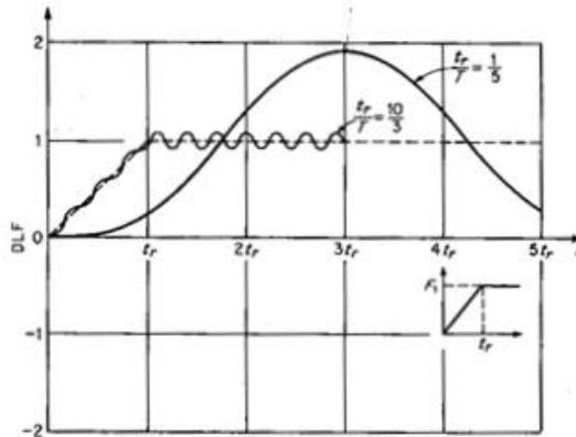
Figure 3. Typical responses of one-degree-of-freedom systems exposed to a constant load with finite rise time  $t_r$ , from [3].
