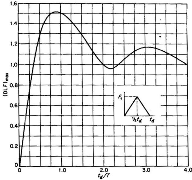
Figure 5 Maximum dynamic response of one-degree-of-freedom systems exposed to a symmetric triangular load with duration  $t_d$  and finite rise time  $\frac{1}{2} t_d$ .  $T$  is the eigenfrequency of the system, from [3].
