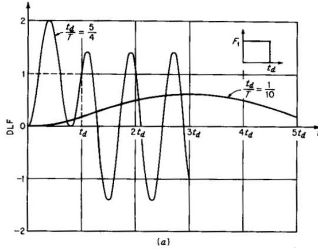
Figure 2. Typical responses of one-degree-of-freedom systems exposed to a rectangular load  $F_1$  with duration  $t_d$ , from [3].
