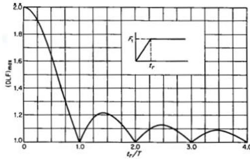
Figure 4. Maximum dynamic response of one-degree-of-freedom systems exposed to a constant load with finite rise time  $t_r$ .  $T$  is the eigenfrequency of the system, from [3].
