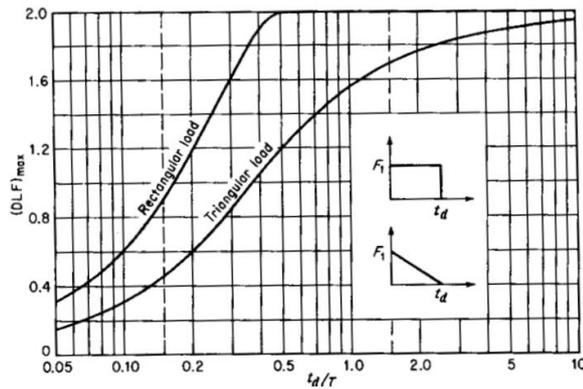
Figure 5 Maximum dynamic response of one-degree-of-freedom systems exposed to a triangular load with duration  $t_d$ . The results are compared with the solution of a one-degree-of-freedom system exposed to a rectangular load with duration  $t_d$ .  $T$  is the eigenfrequency of the system, from [3].
