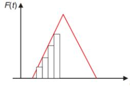
Figure 1. The Impulse loading can be regarded as a sum of rectangular impulses.
