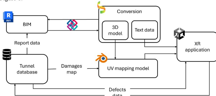
**Fig. 1.** Workflow for XR application development
