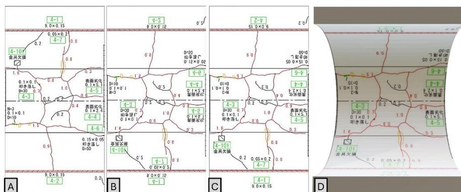
**Fig. 4.** Process for the model texturing on segment 4. In A, the original map of the defects; in B, the mirrored map; in C, the mirrored map with text adjustment; and in D, the map applied to the model.
