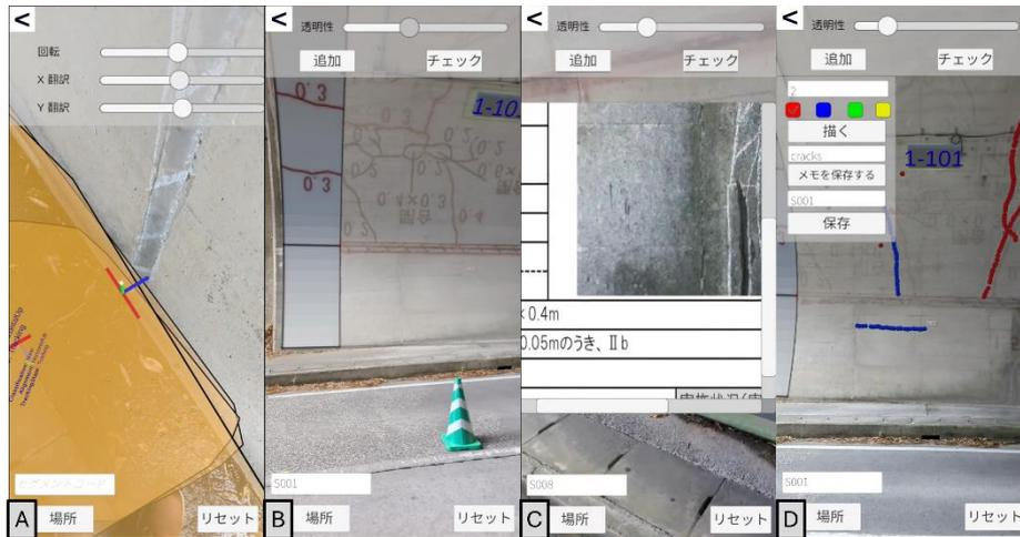
**Fig. 5.** Different features of the application. In A, plane detection for anchoring the model in the real world; in B, the loading of the textured model with transparency changing; in C, the reading of past report of a selected defect; and in D, data collection of new defects data
