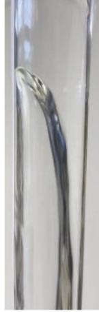
**Fig. 4.** Photograph of the Taylor bubble wedging during bullheading experiments [10].
